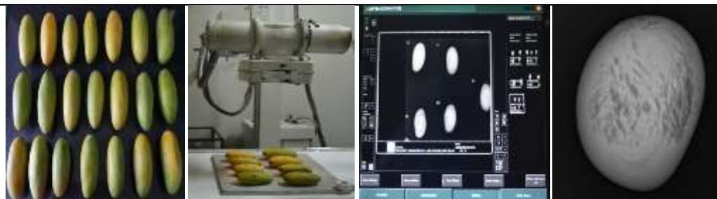
Images showing 1.mango fruits, 2.exposure to X-rays, 3.Image acquisition in computer, 4.X-ray image processing (left to right).
